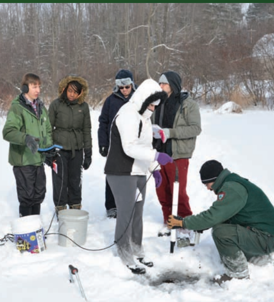
Students and biological sciences faculty at Rice Creek Field Station measure oxygen levels in an iced-over Rice Pond using a Hydrolab Surveyor, used to measure physical and chemical properties of water.
