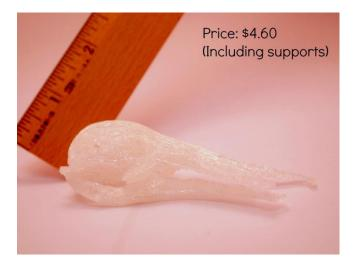
This is from a scan of an actual <u>platypus</u> <u>skull</u>. Because it's an odd shape, it needed printed supports to print correctly. The supports are weighed with the object and count towards the price. They are easy to remove, but we find that needle-nose pliers are helpful.
