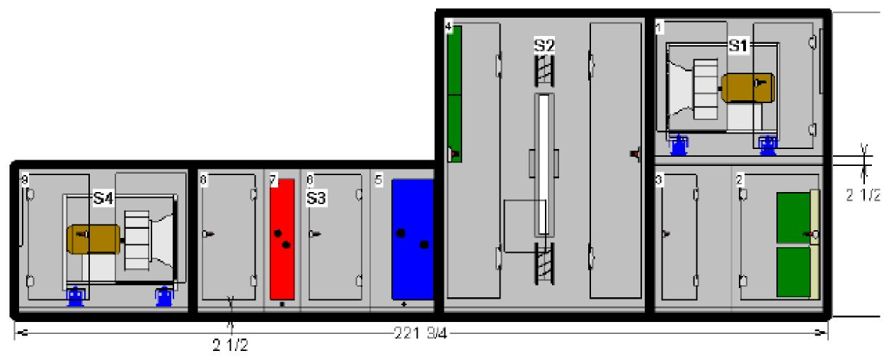
Overall Elevation View: Right - Shipping splits indicated by bold outline. - Measurements in inches
