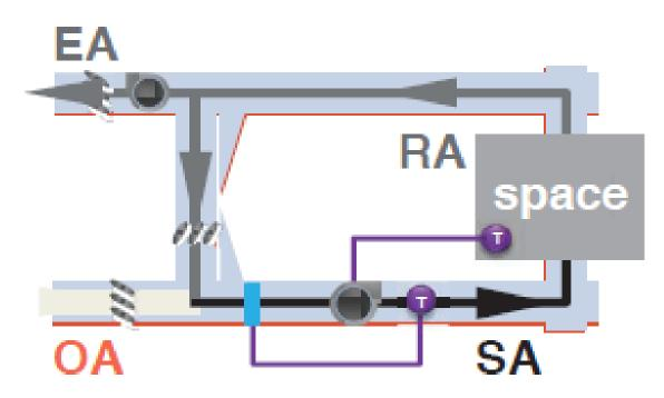
In a Single Zone VAV system, the temperature sensor in the zone is used to vary the air temperature and the air volume in order to maintain the desired set point.
