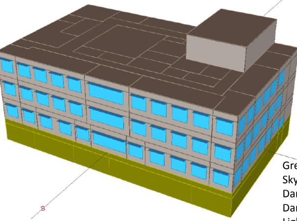
Green : Underground Sky Blue: Windows Dark Blue: Solar Shades Dark Grey: Roof Insulation Light Grey: Wall Insulation
