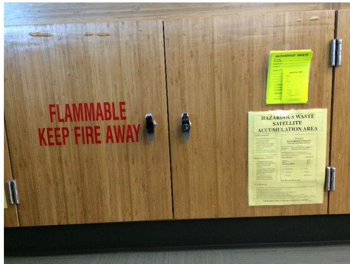
Figure 4: Example Satellite Accumulation Area
