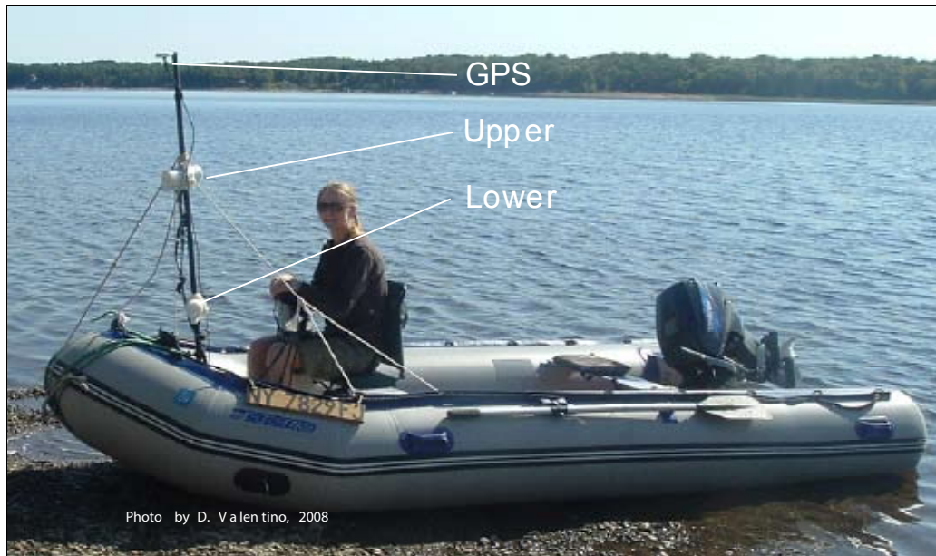
Fig. 4. This photograph shows the inflatable motorboat with the GEM-19GW Walking Gradiometer attached to the bow. The survey required one person to operate the boat, one person to navigate with the GPS, and the one person to manage the gradiometer.
