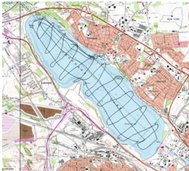
Fig. 3. Topographic map of Onondaga Lake and the surrounding area. The black track shows the path of the magnetic survey.
