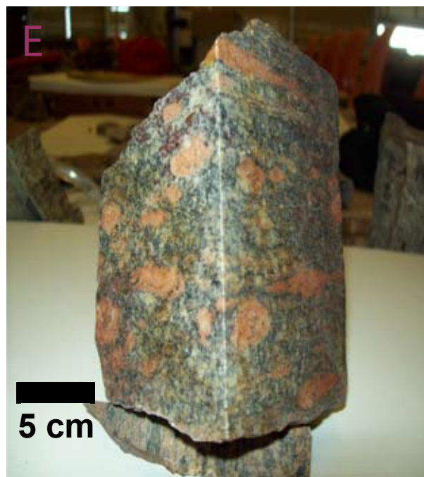
Fig. 6. This sample taken at outcrop PLz 7 in the core of the antiform. It shows a quartzofeldspathic gneiss with excellent L=S tectonite.
