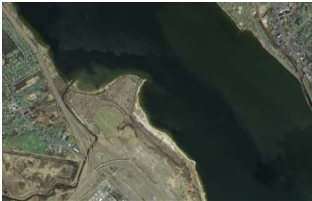
Fig. 6. Air photograph from Google Earth showing the western shore region of Onondaga Lake where Nine Mile Creek flows into the lake. This region is known as the Solvay waste bed and the waste can be seen as a sediment plume along the shore line. This is evidence that the waste bed solids are being dispersed through surface run-off.
