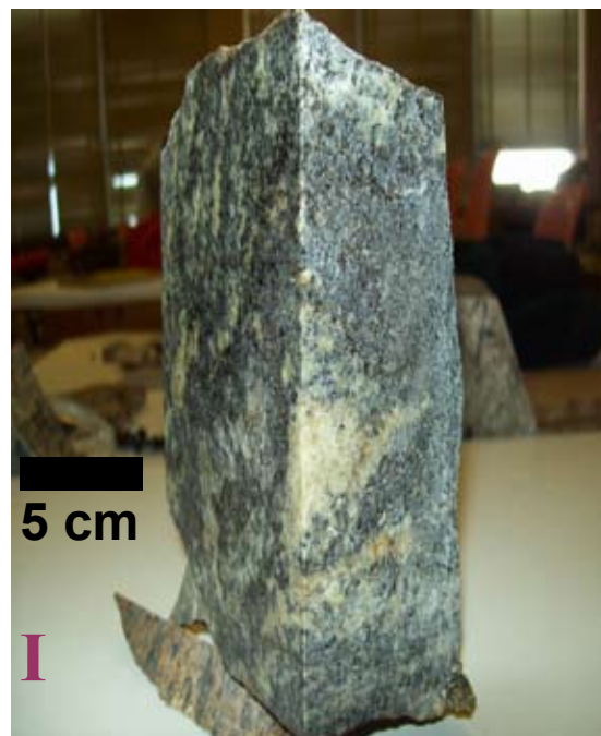
Fig. 11. This sample was taken from outcrop PLz 15, the northernmost outcrop on the North Limb. It shows large grain size and no kinematic indicators, foliation or lineation at all.
