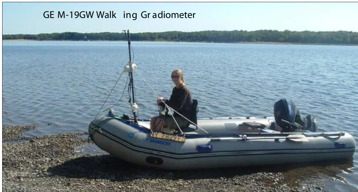
Fig. 3. Photograph of the motorboat with the walking gradiometer attached. Note the distance between the gradiometer sensors and the outboard motor.
