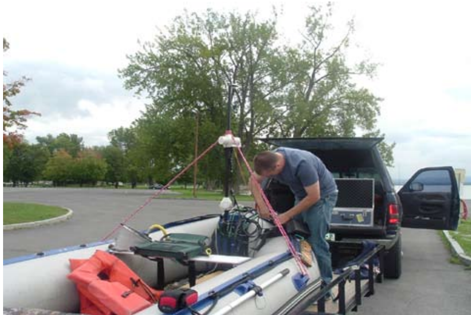
Fig. 2. Photograph of the GEM-19GW Walking Gradiometer being mounted on the bow of an inflatable 14' Sea Eagle motorboat with 18hp, Tohasu outboard motor.
