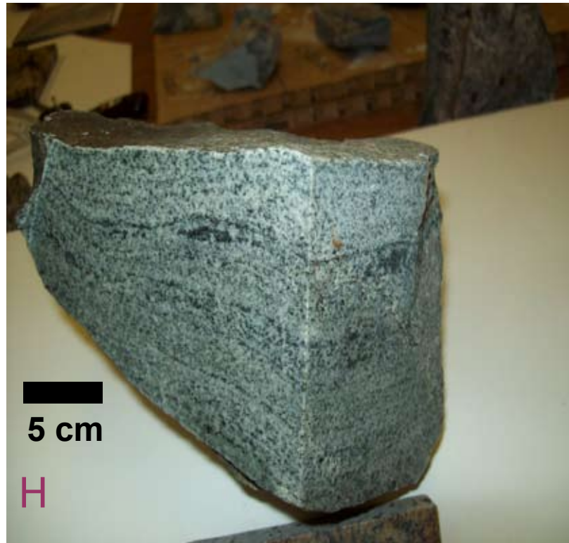
Fig. 10. A hand sample of metasedimentary gneiss with crenulated foliation fabric from outcrop PLz 14 in the North Limb of the antiform. This is an L \ll S tectonite with no sigma or delta clasts.
