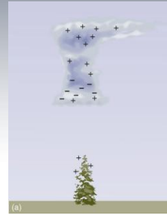
Figure 37A: Charges collect in the base of the cloud
