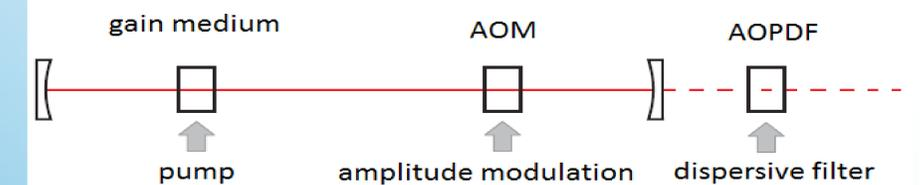
Figure 6: The AOPDF manipulates the higher order phase terms of  $T(\omega)$  to add another phase shift to counteract the original phase shift from the gain medium where  $\omega_g$  is the bandwidth of the AOPDF. This is multiplied by the original electric field and results in a new electric field.
