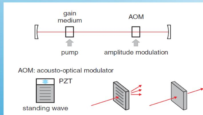
Figure 4: Active mode-locking uses a Piezo-electric absorber transducer that produces a standing sound wave in the material to create different densities allowing for ultra-short lasers to be produced.
