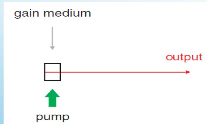
Figure 3: A simple set-up of the laser with the pump which is a green laser, the gain medium that is the Ti:Sapphire, and the output which is a near infrared laser.
