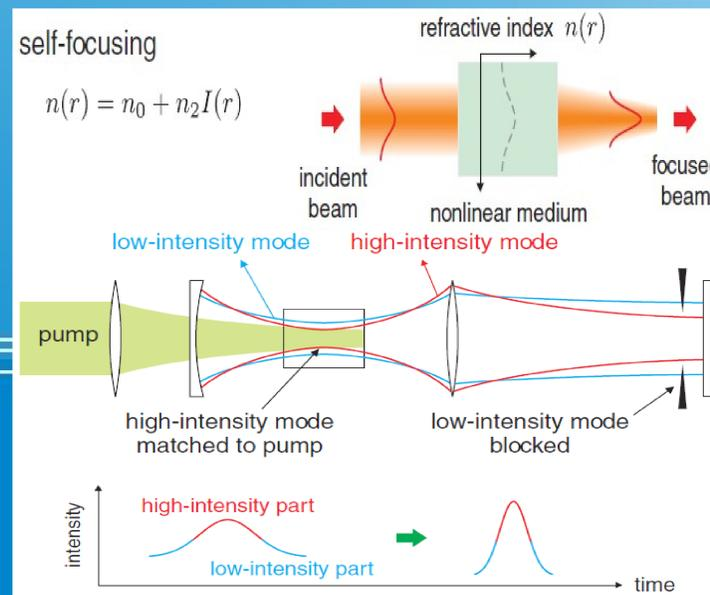
Figure 5: The Kerr-lens mode-locking takes advantage of the non-uniform intensity beam and causes a self focusing effect where  $I(r)$  is the intensity as a function of the beam's radius.
