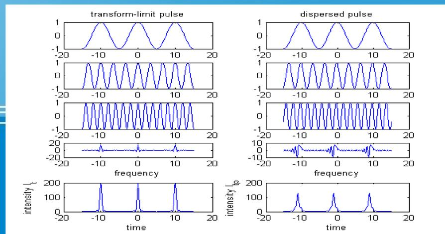
Figure 2: Above are three different frequencies combing into the fourth one down. The left shows a transform limited pulse with zero phase. The right shows when a phase shift is added. Their respective times are shown on the bottom from a Fast Fourier Transformation where the time increases and the intensity decreases with the phase shift.
