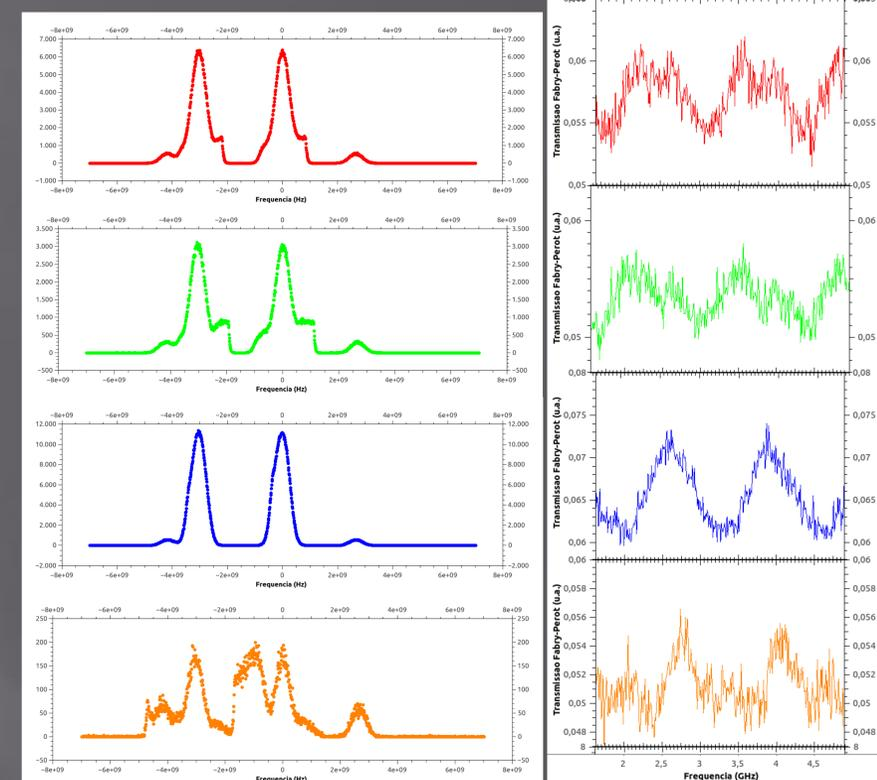
Fig. 3 – ~2 periods of the frequency redistribution are shown (at right, experimental) for the case of laser frequency tuned to resonance and for 2 slightly-shifted frequencies in each direction. Simulation results (left) show the expected result on the curve centered at  $f = 0$  GHz for each case
