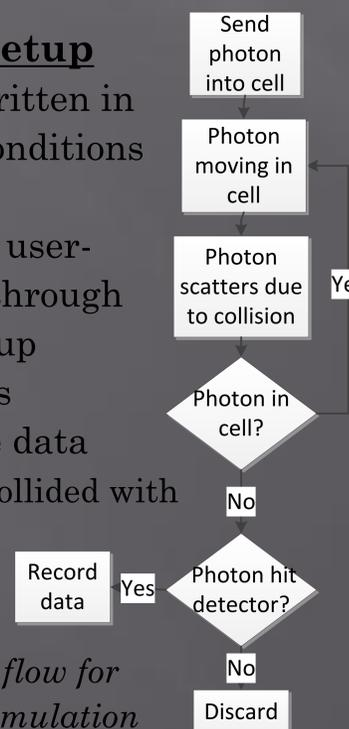
Fig 2. – Basic program flow for Monte-Carlo Simulation
