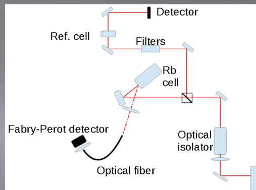
Fig. 1 The experimental setup, containing both a linear absorption reference cell and the main atomic vapor cell
