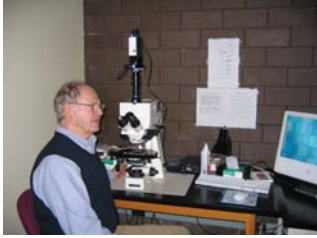
Waiting for an image on the screen at the Zeiss Axiophot Epifluorescence microscope, digital camera, and computer in Carol Peterson's lab at the University of Waterloo, Ontario.
